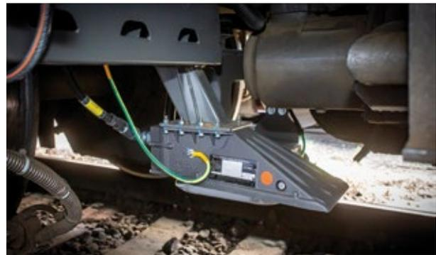
*ETCS sensor DRS0551 on a 362 series locomotive*
